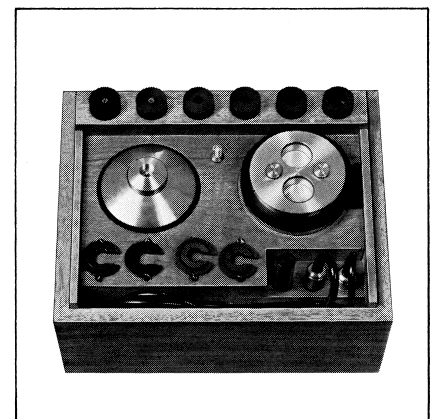
Fig.24. High Pressure Microphone Calibrator Type 4221
